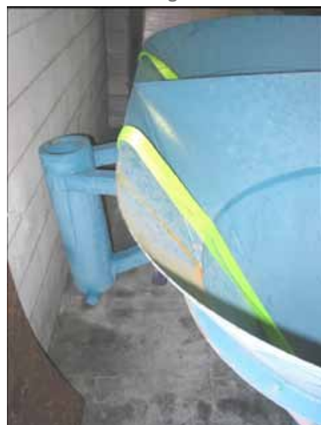
FEEDER HOPPER ATTACHMENT POINT
